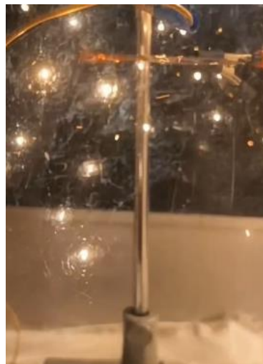
Fig.2 Spheres with a visible diameter of up to 7 mm, realized in a capillary discharge.
